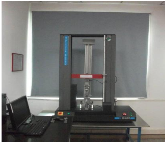
Dual-Arm Tensile Testing Machine
