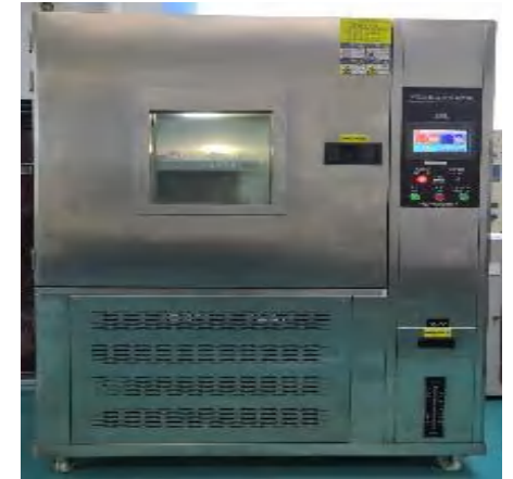
High & Low Temperature Testing Machine
